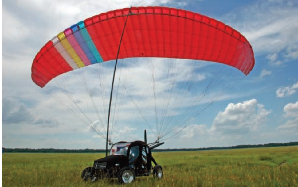
The mast system eliminates unfolding the parachute on the ground, as traditional PPCs do, avoiding the possibility of snagging or tearing the chute on rough terrain and reducing the area needed to unfurl the chute.
