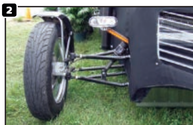
1. The Maverick’s cloth wing stows in a zipped up compartment on the top of the vehicle. 2. The front end suspension and high ground clearance make the Maverick suitable for off-road driving. 3. The Subaru engine that drives the vehicle on the ground and supplies power to the prop in flight is located at the rear of the vehicle.
