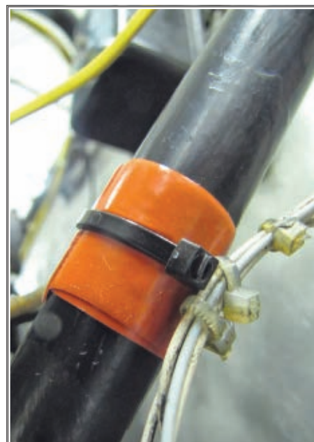
Uniwrap in place under a wire tie.
