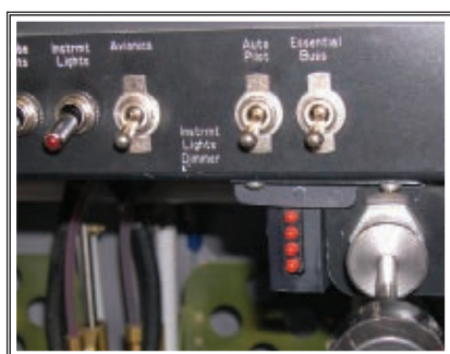
Jerry's assembled circuit board installed on his panel.
