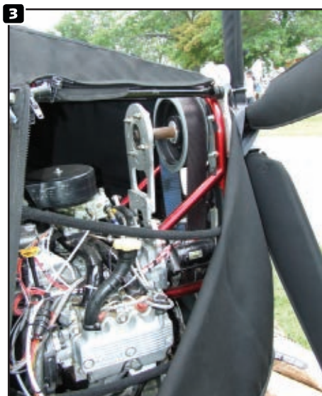
1. The Maverick’s cloth wing stows in a zipped up compartment on the top of the vehicle. 2. The front end suspension and high ground clearance make the Maverick suitable for off-road driving. 3. The Subaru engine that drives the vehicle on the ground and supplies power to the prop in flight is located at the rear of the vehicle.
