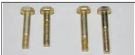
Note the similar color but much longer thread length of the Grade 8 bolt (on the right in each pair) as compared to the AN bolt.
