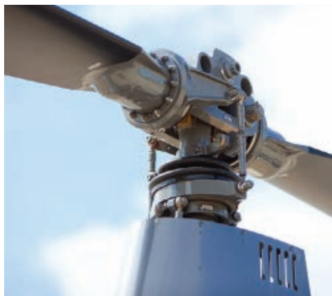
The main rotor is mounted on a vertical mast above the helicopter. The pilot controls the altitude, speed, and direction of the helicopter by using the flight controls to vary the pitch of the main rotor blades.
