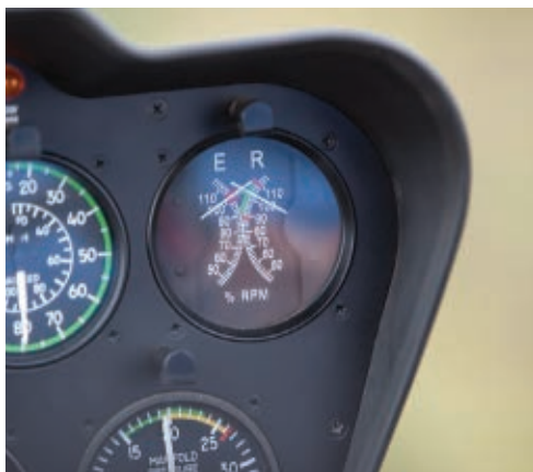
A dual tachometer indicates the engine rpm and main rotor rpm. In normal flight the needles join together and act as one.
