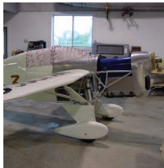
The nose bowl for the cowling was profiled off of the original part, stored in EAA's hangar prior to the restoration of Art's original Jeep for the museum.
