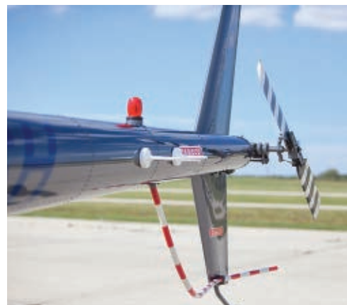
The tail rotor (or antitorque rotor) is controlled by the antitorque pedals and counters the torque created by the main rotor. This prevents the helicopter's fuselage from spinning opposite the direction of main rotor rotation.
