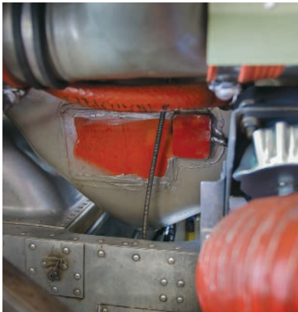
A Tanis heater installed on a Cessna 210.
